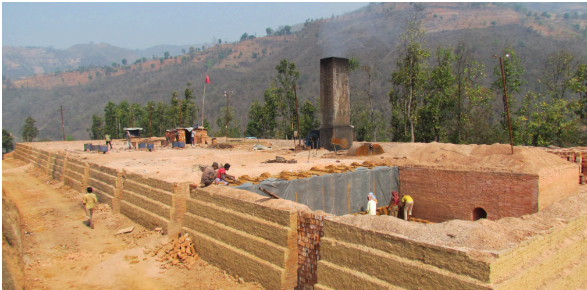
Figure 1: A zigzag kiln in operation. Bricks are covered with a layer of ash, and workers feed coal from above ( Maithel et al., 2014b, p.9 ).
